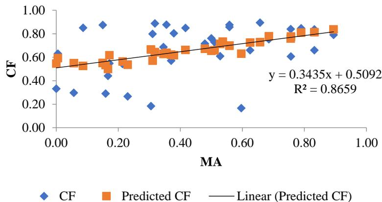
Fig. 2. Capacity factor (CF) in dependence on share of manure (MA) in feedstock
