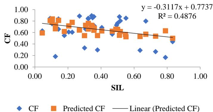
Fig. 1. Capacity factor (CF) in dependence on share of silage (SIL) in feedstock
